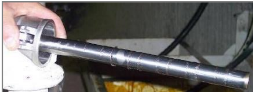
Contaminant captured when an OEI Magnetic Scrubber was installed in a lube shed supply line to test new hydraulic fluid.
